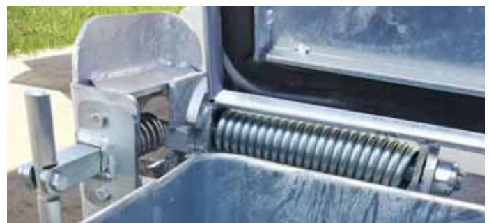
Lid locking and lid lightening springs
