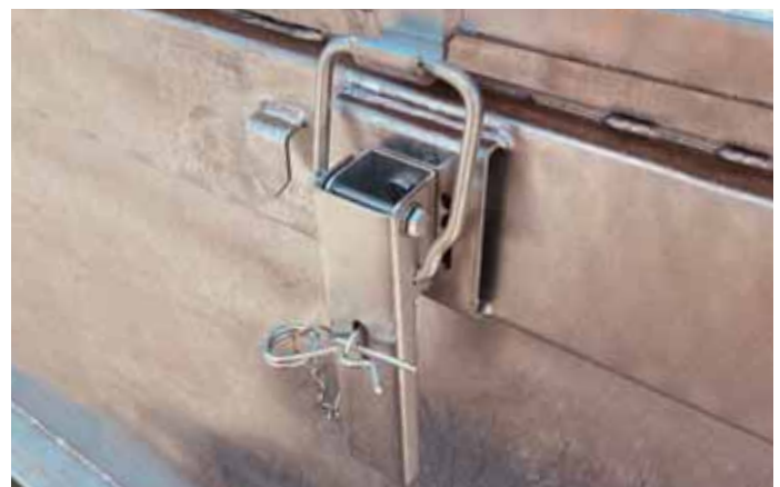
Lid lock - locked and secured
